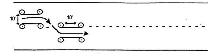
(Distance between barriers is length of bus plus 3 feet ) Width of barrier alley is 10 feet .
